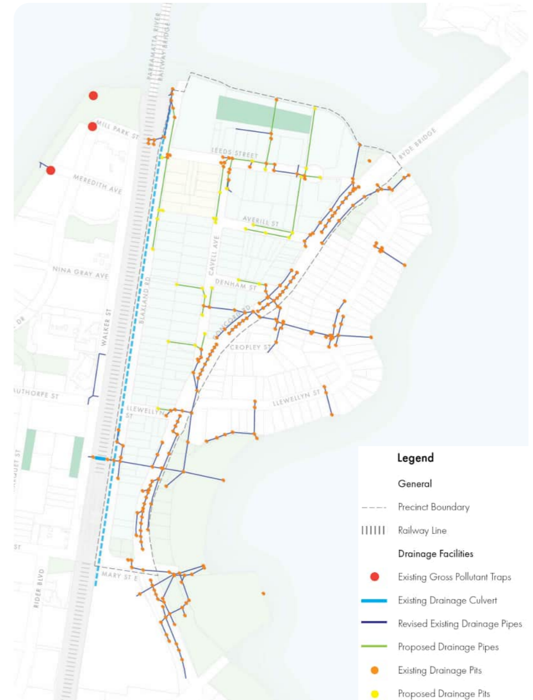
Figure 12. Pits and Pipes Map
