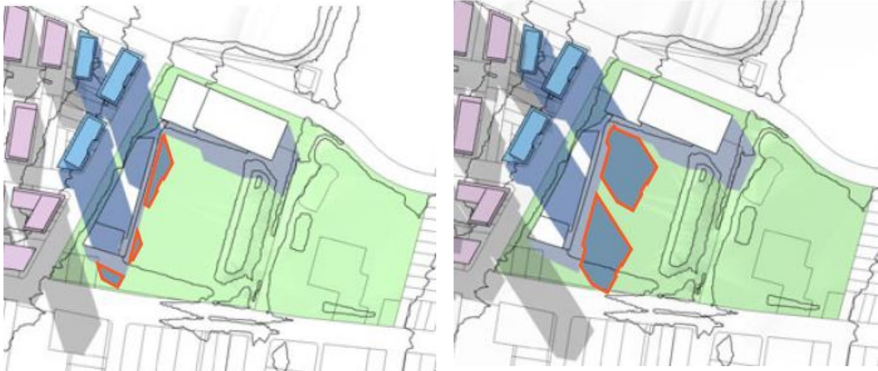
Figure 21: Shadow analysis of subject Proposal at 1pm (lhs) and 2pm (rhs) mid-winter (SGL independent Urban Design Review)
