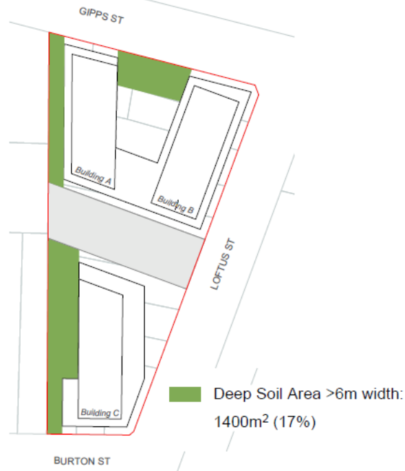
Figure 29: Deep soil calculation of the recommended building layout (SGL independent Urban Design Review)
