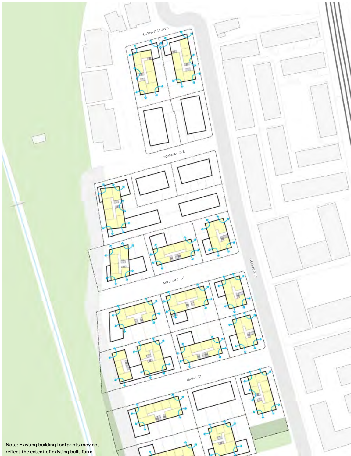
Figure 60: Typical upper level floors - Rothwell Avenue to Mena Street Existing open space Proposed open space Potential site amalgamation Ventilation > 2 hours of Sunlight < 2 hours of Sunlight
