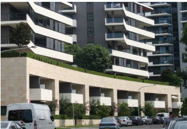
A lower street wall height helps to integrate taller development with lower residential scales
