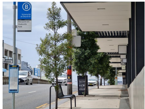
Figure K20-36 Awnings should be designed to allow for street tree planting
