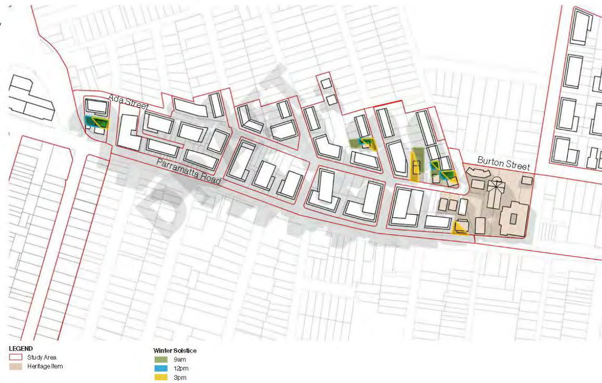
Figure 5.15 Burwood–Concord West: master plan heritage impacts analysis, potential overshadowing to heritage items. (Source: GroupGSA)
